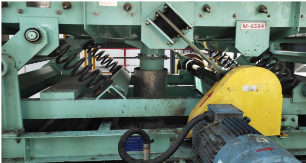
Installation of anti-vibration pads for pumps and vibrators
